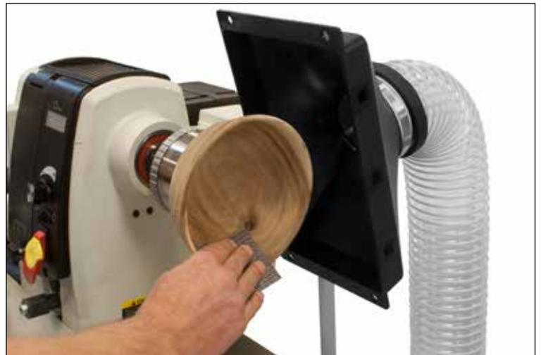
You are now ready to start using your new Big Sweep Dust Collection System. There are many ways to adjust the Big Sweep to achieve the best suction for any project. Your Big Sweep system is designed to pivot, tilt, swivel and slide into any position you need.
