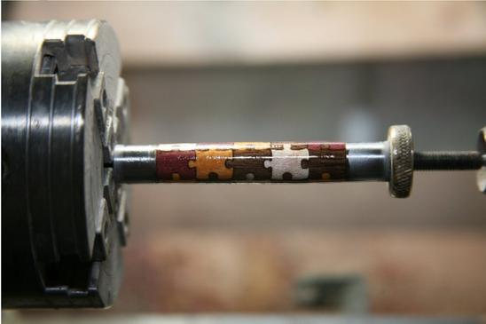
The barrel can now be finished with a finish of your choice. CA glue works great and would provide a great long lasting finish. The pen in this project was finished with CA glue.
