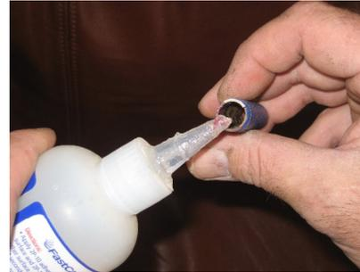
Remove the scuffed brass tube from the assembled puzzle and use any familiar method to glue the brass tube into the assembled puzzle blank. Ca glue works great and cures pretty fast. Make sure that you give the glue enough time to cure before you proceed with the next step.
