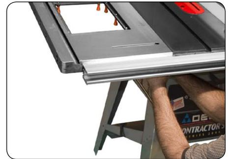
Install the bolts while a friend holds the table in position. Just snug the bolts for now. Make absolutely certain both surfaces are smooth, flat, and free of burrs before mating the two tables together.
