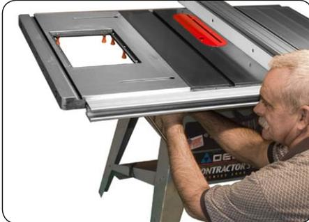
Tighten the bolts gradually and evenly. Use a soft tipped mallet to lightly tap the table surfaces. If your router table is not flat with your table saw's table, you may need to shim it.
