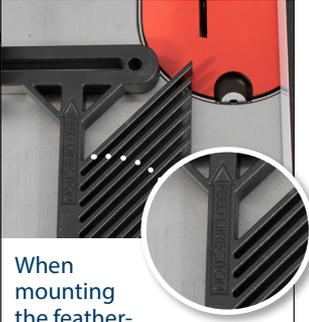
When mounting the featherboards, always make sure that the "FEED DIRECTION" is pointing toward the cutter. This will make sure the fingers of the featherboard will work properly
