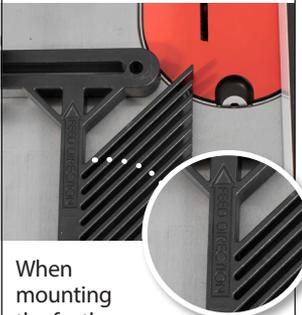
When mounting the featherboard, always make sure that the "FEED DIRECTION" is pointing toward the cutter. This will make sure the fingers of the featherboard will work properly
