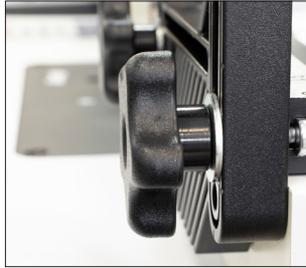
With the the supplied T-Bolts (8) installed on to a single featherboard, slide the t-bolts into your track. Position the featherboard to your desired location, Place slight, equal pressure on the featherboard toward the stock and fence and secure the knobs.
