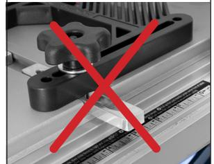
Some table tops may not be large enough to handle this featherboard system. The featherboard must always be sitting flat against the table with no overhang of the miter bars. If there is overhang, DO NOT USE the featherboard on that table top.
