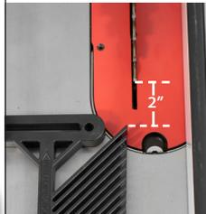
Always make sure that the last finger on the featherboard is at least 2" in FRONT of the blade or cutter on the in-feed side. This ensures that the stock will not "pinch" against the blade or cutter when feeding your stock through.
