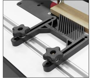
With the supplied T-Bolts the featherboard can be attached to a standard mini style track. You can find these styles of track on many router and some table saw fences and you will also find them embedded on many router table tops. This provides you with the flexibility to use the featherboard on many different workshop machines.
