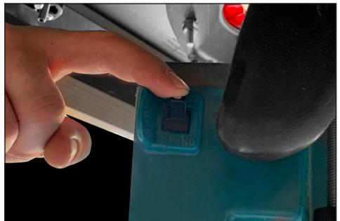
Turn on the switch to your power tool. If everything is setup properly your power tool should NOT turn on.
