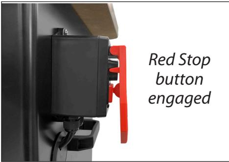
The reason nothing happened after turning your power tool switch on is because the large red stop sign paddle and button are still engaged.
