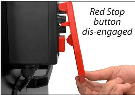
To enable the green start button, lift up on the stop sign paddle to disengage the “red stop” button.
