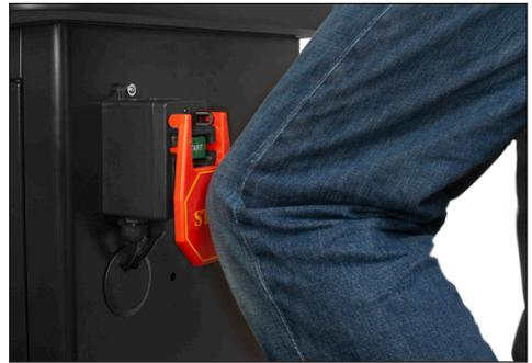
To turn the power off, simply bump or press the large red stop sign paddle.
