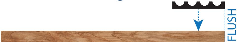
On one of the 2" x 4" ripped halves, use the 1/4" Wood Screws (6) to secure one of the 6 3/4" notched bars (1) flush to one end as shown above.
