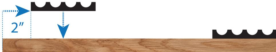
On the other end of the ripped half, measure in 2" from the end and secure one of the notched bars (1) at that mark.
