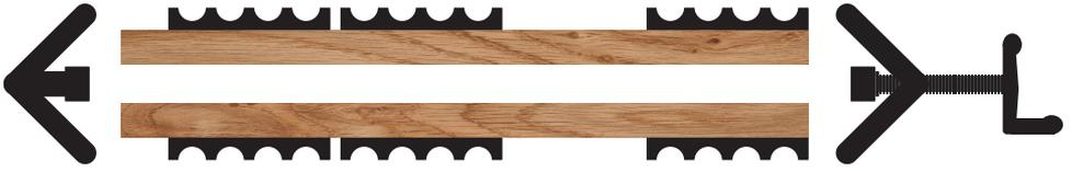
Once the wood bars are complete, they should resemble the image above and are now ready for the clamp assemblies to be attached.
