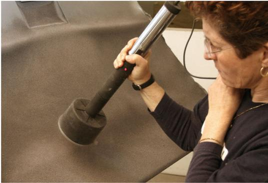
Hold the electrostatic applicator 4" to 5" from the surface being coated. Slide the switch forward and depress button until you see the red light go on. Gently rock the applicator to assure the flocking fibers continue to flow into the static field. Slowly move the applicator around the piece.
