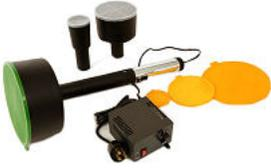
Remove the screened cover and fill no more than  $\frac{3}{4}$  full with Suede-Text flocking fibers. CP 70 Check that your transformer is plugged in and set at the correct voltage. This will usually be at 70kV. Press the "on" button to make sure the flocking fibers are flowing before beginning your coating job.
