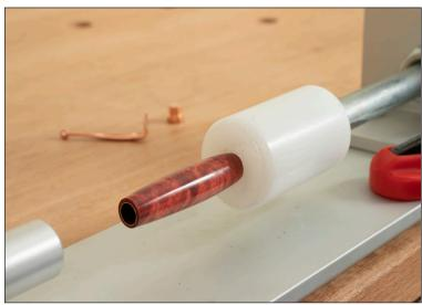
Once in place hand press the cap and clip onto the barrel. Next, slowly press the parts together by pushing the handle lever toward the pen. This pushes the aluminum stop towards the UHMW stop. Continue this motion until the cap and clip is pressed up against the top of the barrel. Finish assembling the pen and check all the mechanisms to make sure they are working properly.
