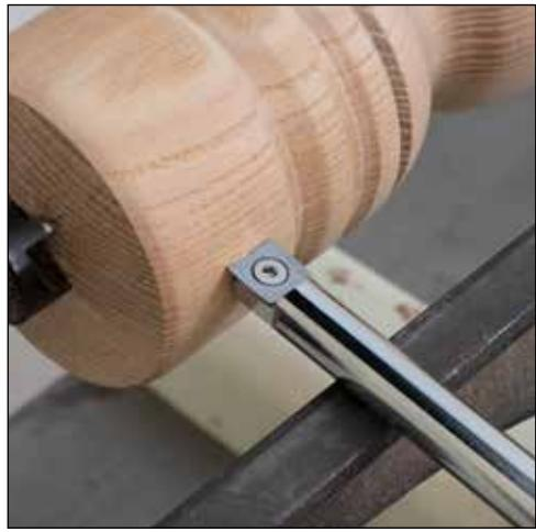
Use the square cutter when you need to remove larger amounts of material. Ideal for flat surfaces and works especially well working or turning pens
