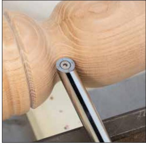
The round cutter is ideal to be used on concave and convex surfaces as shown above. Works exceptionally well on curved goblets, tops and more.
