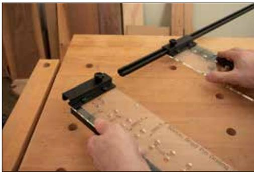
Loosen the studded round knob at the top and bottom of the jig templates. If installed, remove the M4x3/16" Socket Head Stop Screws and Washers ( Parts 1 & 2). Slide the jigs off of the long track rails.
