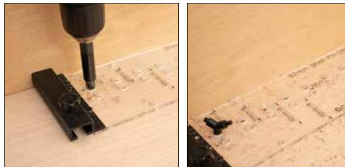
Drill the first hole at the bottom of the jig with the appropriate drill bit (either 1/4" or 5mm drill bit – both are included). Once the hole is drilled. DO NOT drill anymore holes until you continue to the next step
