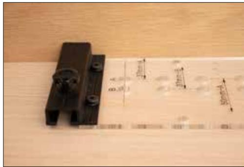
Place the acrylic jig template on top of your mark and line up to the center of the pre-drilled hole. Make sure that you are using the appropriate side of the template for your setback. In this example we are working this project using the 37mm setback, so that edge is up against the corner of the cabinet.
