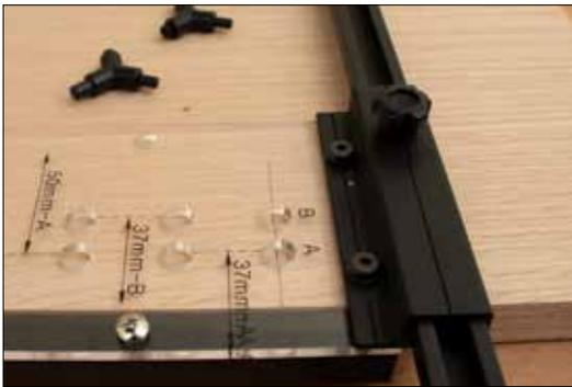
With the shelf pin jig fully assembled, place the jig onto your stock and close both sides of the jig up against the sides of your stock piece. Lock the jig by securing each of the round knobs securely. Align the jig with the first hole on the bottom of the jig as shown here. Make sure both sides of the jig properly align with the marks made in the previous step.
