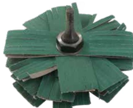
Once all the abrasive strips are on the mandrel, place the steel washer on to the last set of abrasive strips and firmly push it down. Secure the mop using the supplied nut. The nut is has a reverse thread to keep the mop secure while in use. Secure
