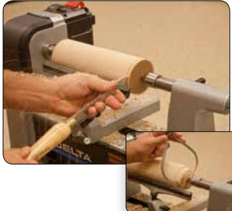
Cut a minimum 5/16" long tenon to fit into the lathe chuck jaws. Use your calipers to make sure you have the correct size of the tenon.
