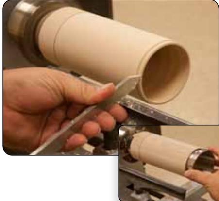
For the lip of the mug, turn a 1/4" rabbet on the top of the blank (with lathe power off). Check as often as possible to ensure a proper fit with the stainless steel insert. (see step 13)
