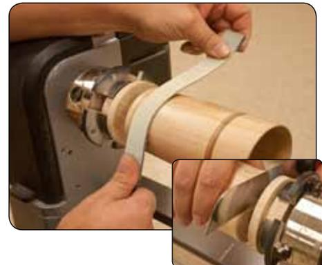
Sand the mug through 320 grit. Finish the parting cut at the base to about 1" in dia. The cut is typically made at a slight angle to give you a slightly undercut base. With the lathe turned off, remove the mug with a fret saw - sand off excess.
