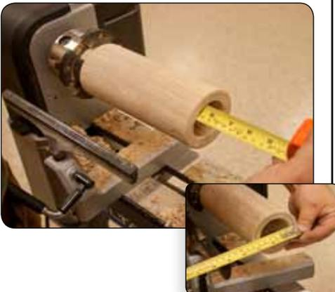
Make sure the depth of your hole is correct and mark a 2-15/16" diameter circle on the open end of the blank. This is your finished inside diameter of your wood sleeve.
