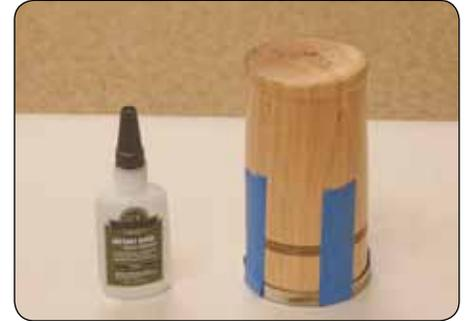
Slide the mug into the blank until it sits properly inside and remove any excess glue. Secure the mug while drying and flip upside down - allow to dry.
