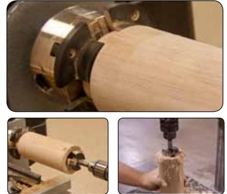
Mount the blank into your lathe chuck using the tenon cut end. Drill a 5-3/4" deep hole into the blank using the 2-1/8" forstner bit. Be sure to clear the debris and chips as often as possible.
