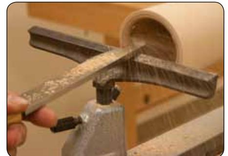
With a heavy scraper or hollowing tool, turn the remaining portion of the inside of the blank so it matches the taper of the beverage mug.
