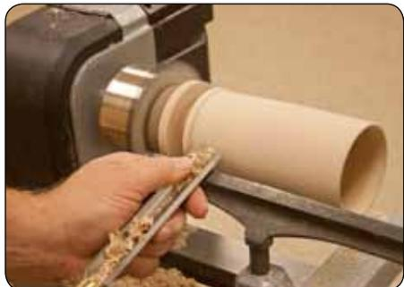
Turn your blank to shape. Make sure you leave a shoulder on the top side for the mug to register. This provides a nice, clean transition from the stainless steel to the wood. Remember, the mug shape can be any shape or design. Add your own finishing touches!
