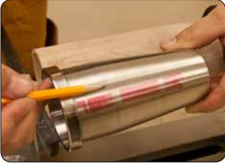
To achieve a nice final fit, mark the outside of the mug insert with a dry erase marker. Once marked (with lathe power off), you simply press the mug into the opening while twisting. Missing ink on the mug will show areas that still need to be turned. Repeat this process as needed.
