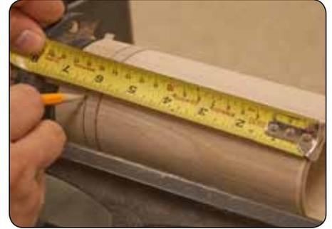
Measure the depth of your hole in the blank. Add a minimum of 3/8" to the depth and make a mark on the outside of the blank. (This measurement includes the lip of the blank)
