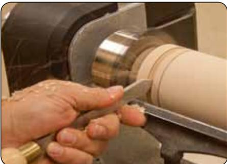
With the parting tool, start a parting cut on the left side of the mark to about 1/2" deep. This is your reference to the bottom of the mug. (see diagram on page 4)
