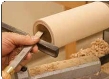
Working from the open end, turn the upper portion of the sleeve flat to the 2-15/16" diameter mark approximately 1-7/8" into the sleeve.
