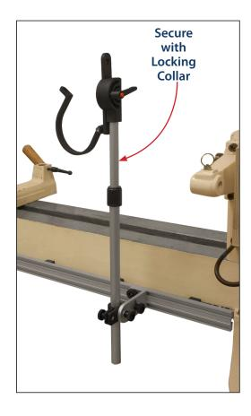
**Step 10**Attach Top Assembly to Base Assembly
