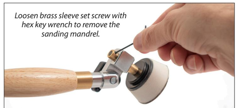
*Loosen brass sleeve set screw with hex key wrench to remove the sanding mandrel.*
