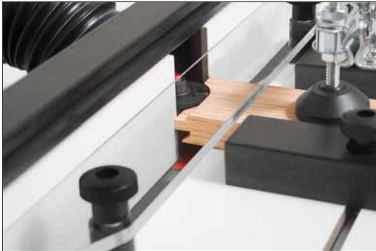
14. If necessary, repeat the router bit height setup process until the stile and rail mate perfectly as shown below.
