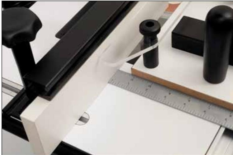
3. With the 4 cap nuts on the toggle and the rear post knob loose, keep the Clear Acrylic Fence Guide against the router fence, use a square to set the Fixed Fence to 90° in reference to the Coping Sled Base. Once you have the Fixed Fence set, firmly secure the rear Post Knob Handle.
