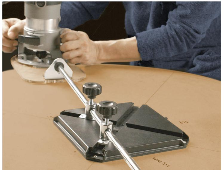
With the power turned off, move the router around the ellipse before turning it on to be sure that its tracking properly. Plug in the router, turn it on and plunge the router so the bit cuts the full thickness of the board. Slowly work the router around the ellipse in the counter clockwise direction. Working the router in a counter clockwise direction keeps the router from pulling away from you while cutting. For thicker stock, you may need to make multiple depth cuts for best results.
