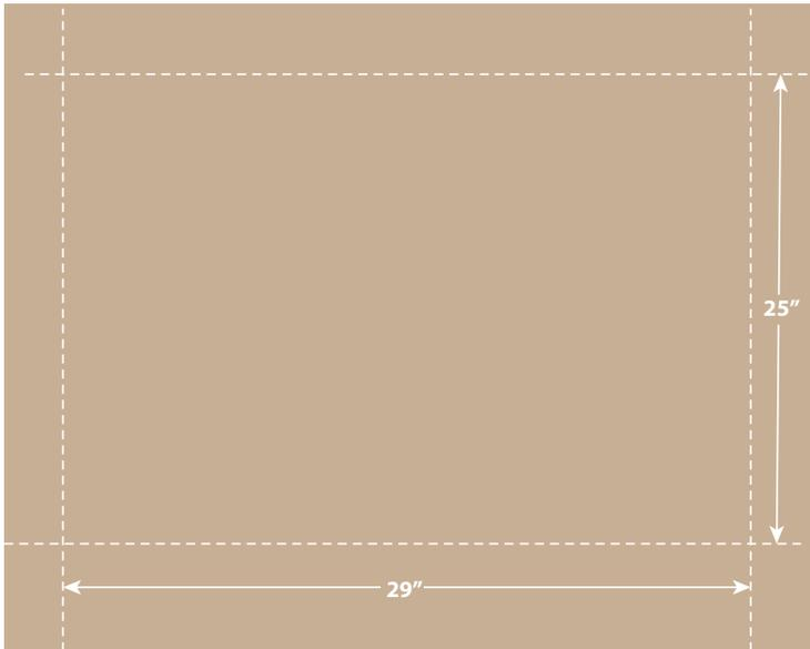
Before using the jig, layout the desired length and width of your ellipse. Generally, this is done on the bottom (underside) of your workpiece.
