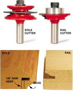
After routing the stiles and rails, a single tablesaw cut creates a piece of retaining molding and a rabbet for the glass. Once the bead has been cut off, the stile fits the end-grain profile made by the rail cutter.
