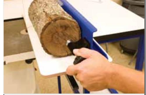
Secure the log in to the mill using the front clamping assembly.
