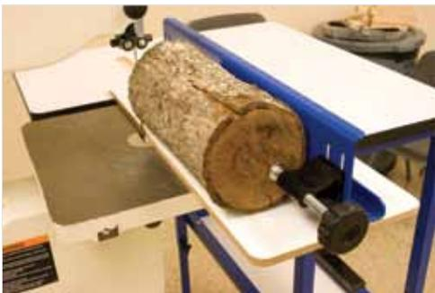
Using the platform as a guide, adjust the log and fence to maximize the yield of the log.
