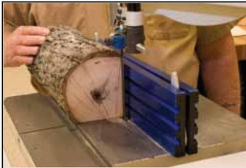
Set up a re-saw fence to your desired board thickness (Carter Mag-fence Shown but not included).
