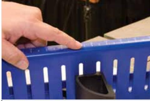
Adjust the back locking jaw to the appropriate mark on the scale.
