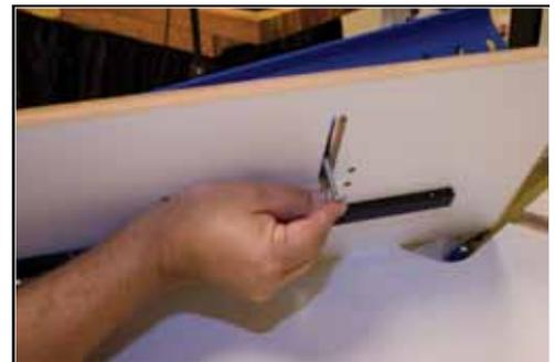
Insert the t-bolts into the platform slots. and mount the log mill fence.
