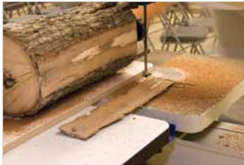
Before making your first cut, make sure the guide assembly of your bandsaw will not impede your cutting progress.
