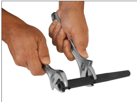
Choose the extension length you would like the Long Bore to reach. With the locking screw removed, thread the rods together and tighten with two wrenches as shown above.
