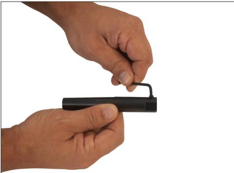
Before threading the extension rods together, remove the locking screw. Failure to do so may damage the threads of the rods and void any and all warranties that apply.
