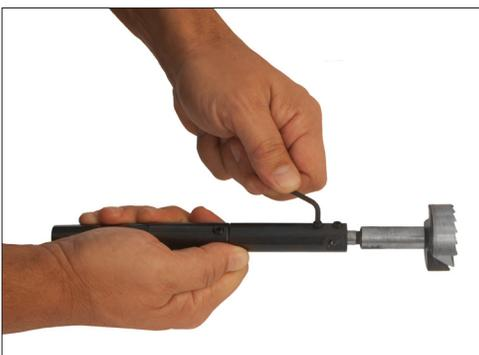
Once you are setup for your desired length, insert your choice of forstner bit in to the forstner bit holder (the rod with two set screws). Secure the forstner bit by tightening to two set screws using a hex key wrench.
