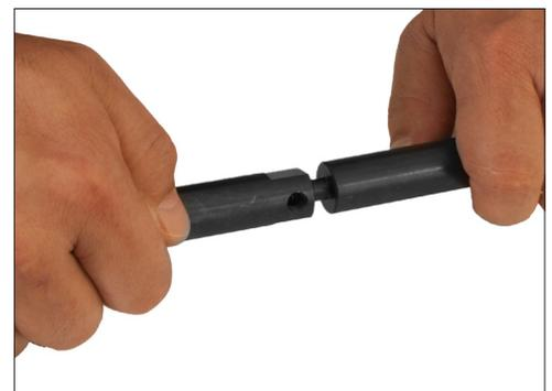
When your finished using the Long Bore rods, remember to remove the locking screws before dis-assembly. Failure to do so may damage the threads of the rods and void any and all warranties that apply.
