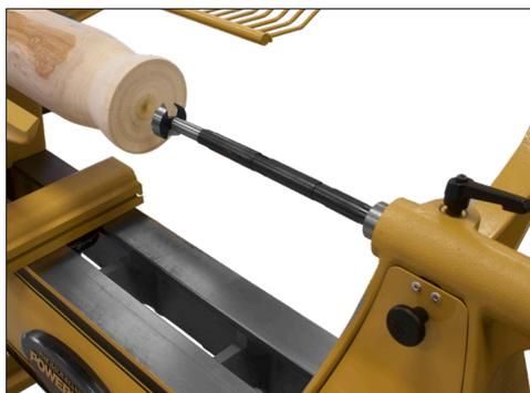
Insert the assembled Long Bore rod with the #2 morse tapered end into your lathe tailstock. With your project mounted on your lathe, turn the lathe on (appx. 800-1200 rpm depending on size of the forstner bit) and slowly feed the forstner bit into the center of your stock piece.
