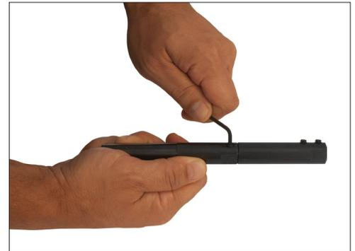
Once the rods have been tightened with the wrenches, re-insert the locking set screw into rod hole and secure. This is done to prevent the rods from loosening during use.
