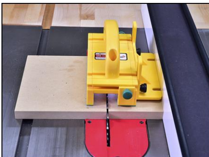
4. Rip a piece of \frac{3}{4} " MDF to 4" wide. Do not move the fence until after Trimming (Step 8) is complete. Note: MDF is better than solid wood or plywood for this application.
