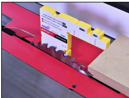
5. Place the MATCHFIT Setup Gauge next to the blade. Raise the saw blade to the center of the notch.
