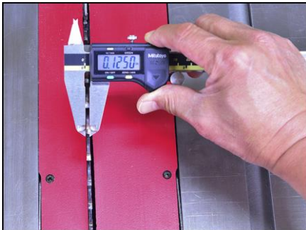
1. With your table saw unplugged, measure the width of the carbide teeth.
