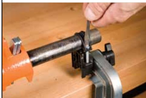
Remove one of the screws from the harness clips on each of the Maxi Clamps. Rotate clip out of the way, and set pipe clamp onto the harnesses. Rotate the clips back over the top of the pipe and secure as shown in photo above.
