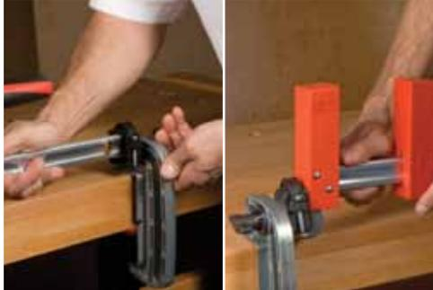
Remove the foot clip from your K-Body clamp. Push the steel bar of the clamp into the harness as shown above (left). Now place the head of the K-body clamp onto the steel hooks on the other Maxi clamp. Note you may have to loosen and adjust Maxi clamps for a proper fit.
