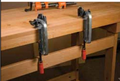
Secure the two Maxi clamps to your benchtop or table top. Have the two clamp harnesses positioned on the top side of Maxi Clamp as shown in photo above.
