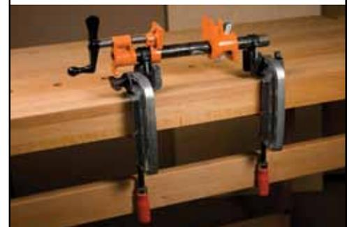
Secure the outer position knobs on both clamps and you are ready to use your pipe clamps for sanding, planing, carving and more.
