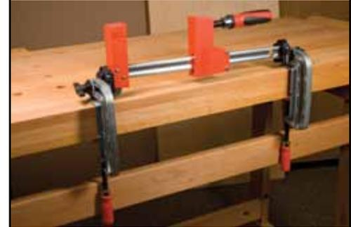
Secure the outer position knobs on both Maxi clamps and you are now ready to use your K-Body parallel clamp for sanding, planing, carving and more.
