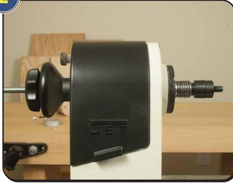
Install the black washer and thread the knob on to the thread of the drawbar and secure. *NOTE: The draw bar is intentionally made extra long to fit most any lathe. You may cut the bar shorter if desired.*
