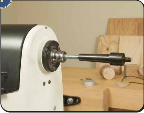
Insert the MT-2 mount into and through the headstock spindle on your lathe.
