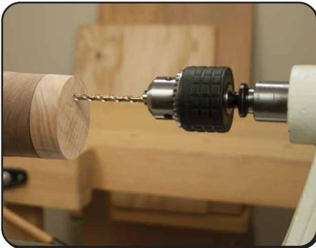
Mount a lathe drilling chuck to your lathe tailstock. Insert a 1/4" drill bit into the chuck and secure. Drill the hole.
