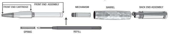
NOTE: Please do not press the front end of this kit with the tip removed. If you do so the parts will not assemble properly and you will void our warranty
