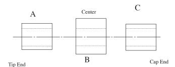
Tip Bushing: A .347" Center Bushing: B .440" Cap Bushing: C .330" Inner hole: .248"
