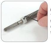
**NOTE:** The wrench comes pre-assembled with an assist spring. This spring is rated to lift most of the weight of the PC-7518 motor. The spring eliminates the need to hold down the plate while making course adjustments. The spring can be easily removed by simply loosening the small set screw in the white plastic foot.
