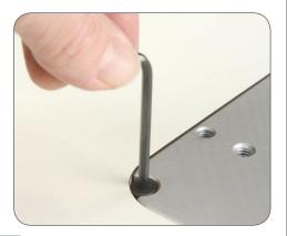
The PRL-V2 also features a brake. For most routers, the brake isn't necessary. However if you experience vibration while routing, the brake will prevent the bit height from changing on its own. A 1/8" hex key is supplied for the brake. **DO NOT OVER TIGHTEN THE BRAKE.** A little pressure is all that is required.
