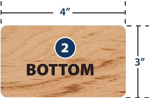
2. Cut a piece of lumber - that is 4" x 3" and at least as long as the Panel Max Slide Rail.
