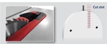
If your saw has a built in splitter or riving knife you need to cut a slot at the rear of the insert. Trace the outline of the slot from your original metal insert, and cut the slot with a bandsaw or a jigsaw. Leave the bridge between the splitter slot & the blade slot as thick as possible.
