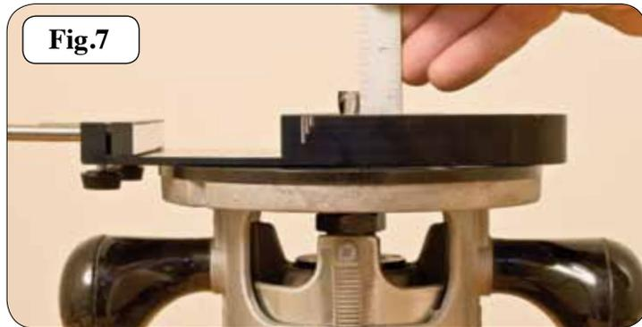
Once you reach your desired depth of cut, lock the height adjustment in place on your router and remove the Dadowiz™ from the router.
