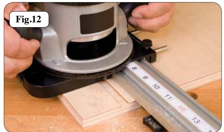
Clean the dado slot free from dirt or debris, and make sure your material fits properly into the slot. If it is too tight or too loose, refer to the "Fine Tuning The Cut" section of these instructions.
