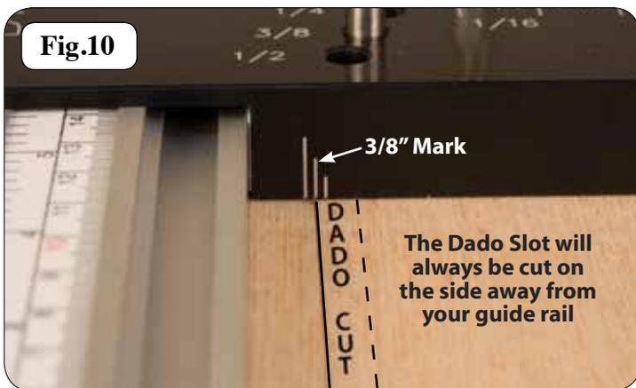
*NOTE: Make sure that the material is supported and will not move around while cutting.*
