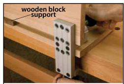
Once your boards are aligned, secure both stock pieces to the jig using the dowel jig knobs.
