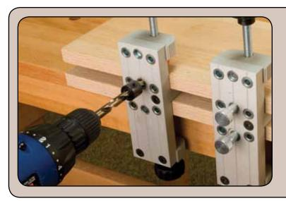
By adding a second Peachtree Dowel Jig (sold separately) you will be able to use the alignment pins, which are perfect for keeping your stock in place while you shift or slide the second dowel jig into position. Once your initial holes are drilled, insert the appropriate alignment pins into those two holes. Now, loosen the second dowel jig and slide it into position and secure. You are now ready to drill your second set of holes. Using a second jig cuts your drilling and setup time in half.
