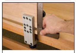
Place the stock pieces to be drilled into the dowel jig as shown in photo above. One board should laying flat, while the other stands vertically. Use a square to ensure the both pieces are aligned correctly.
