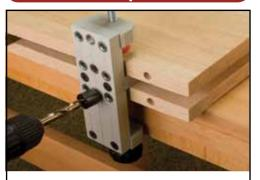
Once drilling is complete, loosen the knobs on the jig. Move jig to the next desired location and repeat steps 1 - 4 of this section until all of your holes are drilled.
