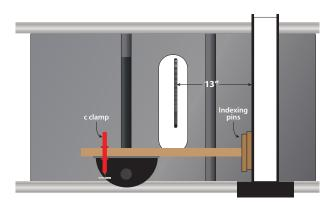
Re-connect the power to your saw. Turn the power on and slide the backer board fence over the blades to cut a notch directly into the backer board fence. Turn the saw off and wait until it comes to a complete stop. Slide the miter gauge and backer board fence back over the blades to its original starting postion. Loosen the c-clamp and slide the backer board fence up against the tablesaw fence and re-secure with the "c" or "f"-clamp as shown in the image below.
