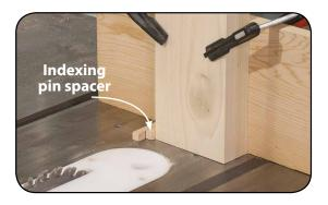
Remove the indexing spacing tool before making your next cut. Turn your tablesaw on and with a smooth forward action make a notch cut through the stock.
