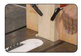
Turn your tablesaw on and with a smooth forward action make your first notch cut through the stock and the jig iteself.
