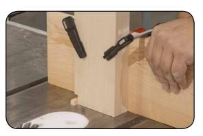
Turn the saw off and wait until it comes to a complete stop. Loosen the clamps and place the two boards onto the indexing pin in the notch cut you just made. Repeat this process all the way across the entire width of the stock until it is complete. Repeat this entire process on the opposite end of your front and back pieces. Your box is now ready for assembly.
