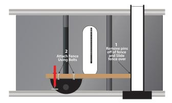
Disconnect the tablesaw from its power source. Most miter gauges have pre-drilled holes for mounting subfences to them. If your gauge does not, you will have to drill mounting holes into it. Secure the backer board fence to the miter gauge through the mounting holes using screws or bolts, making sure the head of the screws or bolts do not protrude past the face of the fence.
