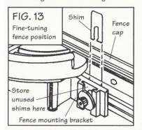
In general, to raise any miter setting to one of the fractions of a degree shown on the chart, add the required shims:
