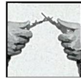
2. Flex belt farther, twist tab 90° and insert tab through end link with thumb.
