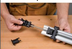
Slide the entire clamping assembly and steel clamp rod back onto the clamp body.
