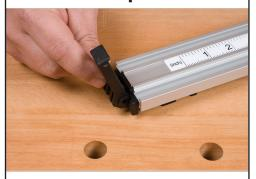
Make sure handle is in the upright and unlocked position.
