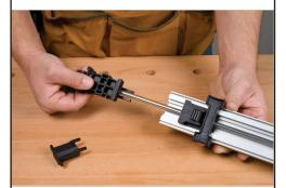
Slide the entire clamping assembly and steel clamp rod from the clamp body.
