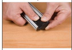
While firmly holding clamp, push the end cap out, up and off the clamp body.
