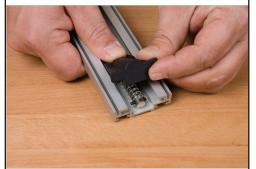
Slide the spring to the end of the clamping rod against the pin.
