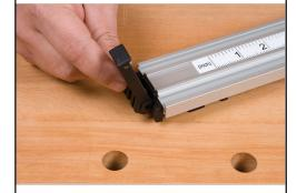
Make sure handle is in the upright and unlocked position.
