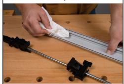
Clean the clamp with a soft cloth and warm soapy water. (Remove any build up of sawdust and glue)
