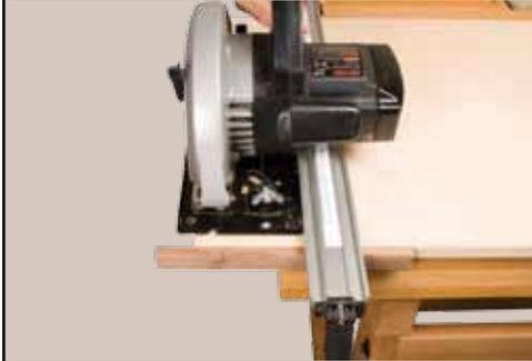
Clamp the PRO-GRIP™ clamp with the story stick attached to a scrap piece of plywood securely. Cutting about a 1/4" of plywood material off with your circular saw, follow all the way through the story stick - cutting the end of the story stick off. Your Story Stick is now set-up for your particular circular saw.
