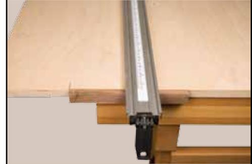
Place a mark on your project stock where it needs to be cut. Place the PRO-GRIP™ clamp with the story stick attached on to the stock. Slide the clamp over until the cut-off end of the story stick lines up with your mark. The end of your story stick shows you exactly where your saw blade will cut through your stock.
