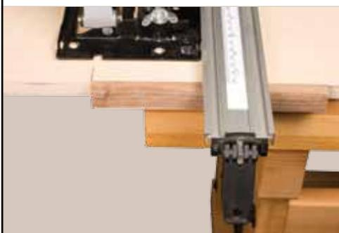
With the PRO-GRIP™ clamp secured in place make the cut on your plywood. The blade should pass right through your mark and right passed the story stick.
