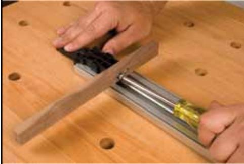
With the pre-drilled countersunk holes facing away from the PRO-GRIP™ clamp jaw, attach your story stick directly to the jaw of the locking clamp head with the two wood screws provided in the pack.
